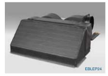
All EBLE configurations are low-profile for installation in height restrictive areas such as beneath a seat or bunk or in overhead spaces. The dual PSC blowers are supported by a sturdy aluminum bracket with cushioned mounts to reduce noise and vibration. Transitional metal surfaces are insulated against secondary condensation and noise. The "positive flow" drain pan is also insulated and lined with anti-slosh, anti-fungal foam.
