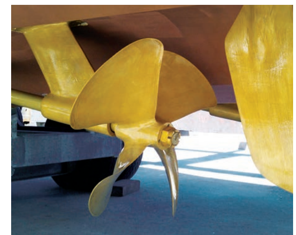
Full PropOne™ application to propeller, propeller shaft and rudder, now ready for immersion
