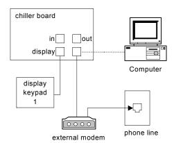
Only one display keypad can be hooked up to a chiller board. A keypad is capable of monitoringand accessing information from the chiller unit.
