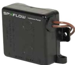
The electronic automatic switch, Ultima Switch uses the patented Mirus field effect detector cells producing micro-electrical fields that detect disruptions caused by water and fluids. Detector cells are totally sealed and are never in contact with the water, will not corrode and are not affected by oil or foreign debris.
