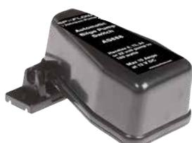
The AS888 automatic float switch has a time-proven micro switch without mercury. When water exceeds the acceptable level, the pump is turned on by a rolling steel ball, which changes the pressure on the micro switch. For fully automatic bilge pumping operation, connect the automatic switch to your bilge pump. The AS888 attaches to any SPX FLOW Johnson Pump bilge pump through a clip on "T-slot" and can be used with 12, 24 or 32V systems.
