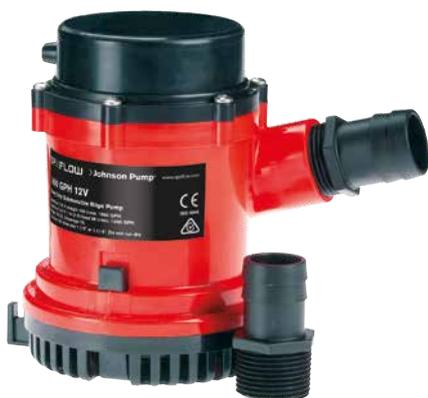
The submersible pumps from SPX FLOW Johnson Pump Marine can handle most bilge pump applications. Heavy duty motors with stainless steel (SS2343/1.4436) shafts and tough thermoplastic bodies provide for a long pump life.
