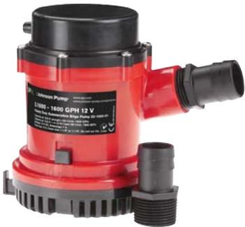
The SPX Johnson Pump Marine submersible pumps can handle most bilge pump applications. Heavy duty motors with stainless steel (SS2343) shaft and tough thermoplastic bodies provide for a long pump life. With an automatic switch installed, the pump automatically starts on when there is water in the bilge and shuts off when it is dry. Salt water tested - salt water tough.
