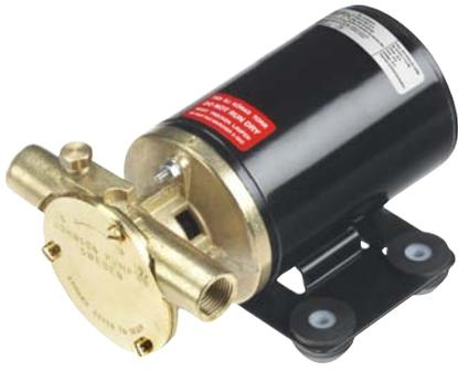
With their high level of flexibility, these pumps are ideally suited for use in boats as bilge and deckwash pumps, fresh water pumps, refuelling pumps for oil and diesel. These pumps may be combined with a vacuum switch for automatic operation. Capacities vary from max 15 l/min to 55 l/min, allowing the proper matching of the pump to the application. All motors are heavy duty to provide long service life even under heavy use. Available in 12 or 24 volts.
