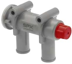
A vacuum valve is a cheap insurance against water intrusion in a engine with expensive repairs as a consequence. The maximum ambient temperature should not exceed 60 °C. The valve opens at a pressure which is equivalent to 3-5 cm Water Column. The materials which are used are resistant to sea water and fresh water, and to glycol compounds in appropriate concentrations. Avoid exposing the valve to oil and grease. If it has been in contact with such substances, please clean or replace it.
