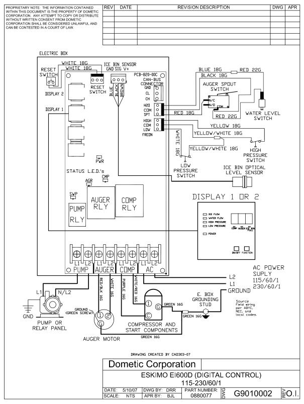
Figure 3. Wiring Diagram for digital control
